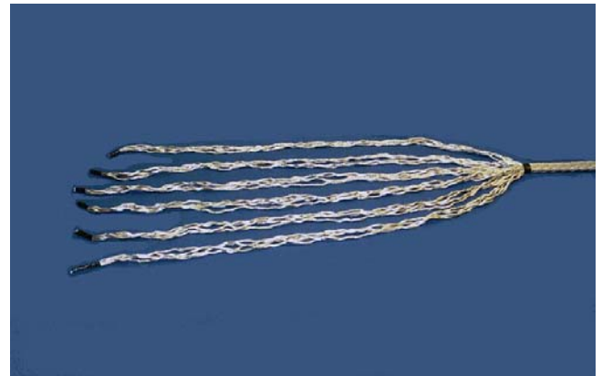
2. Loose up the strand's of the rope and tape two and two together.
