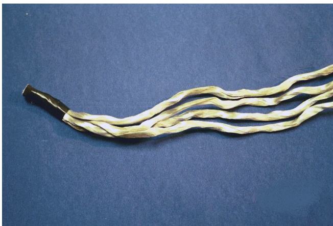
3. The strand's taped together should have same twist direction.
