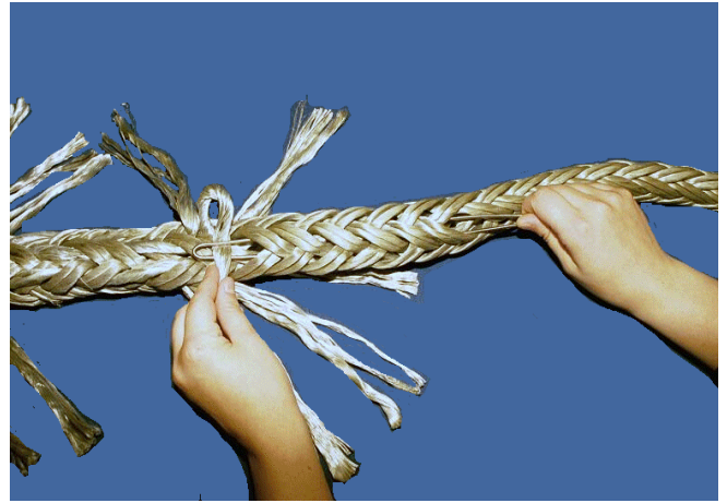
18. The short strand ends are pull into centre of the rope.
