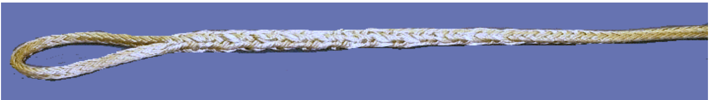
19. The splice is now finished and it should look like this. The tuck splice is absolutely the best splice for Dynex ropes as it will never slip and it gives the highest retaining strength possible to achieve with splice.
