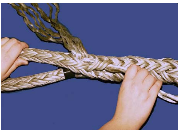
15. The rope is turned over to the other side and the strands spliced into the rope as before.
